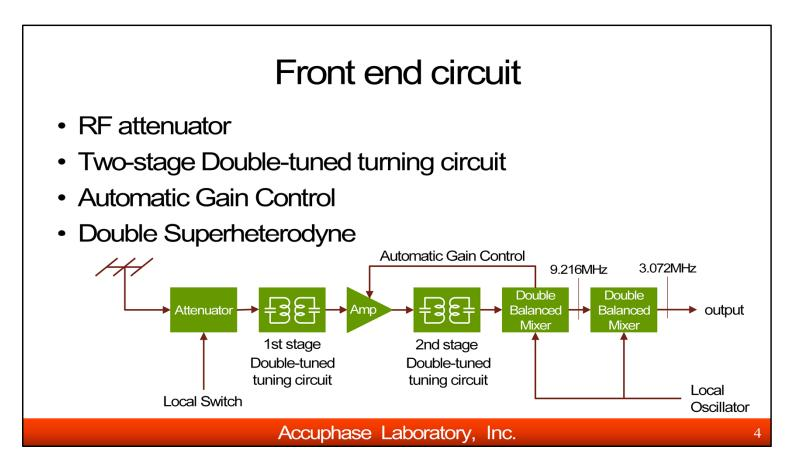
The front end in FM tuner just picks out and amplifies the desired station signal from many others coming from the antenna, and converts it to the intermediate frequency.
