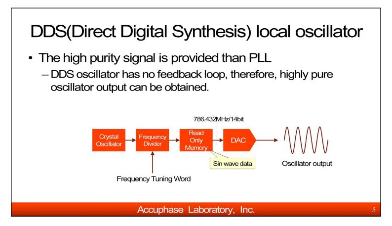
Generally, PLL(Phase Locked Loop) circuit is used for a local oscillator. In a conventional PLL circuit, feedback is used to stabilize the frequency, but this produces frequency modulation components that tend to degrade tuner's noise characteristics.
