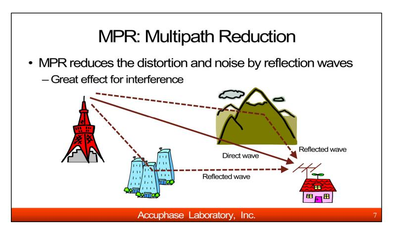
Multipath reception refers to a condition where the same broadcast signal reaches the antenna via several different propagation routes.
