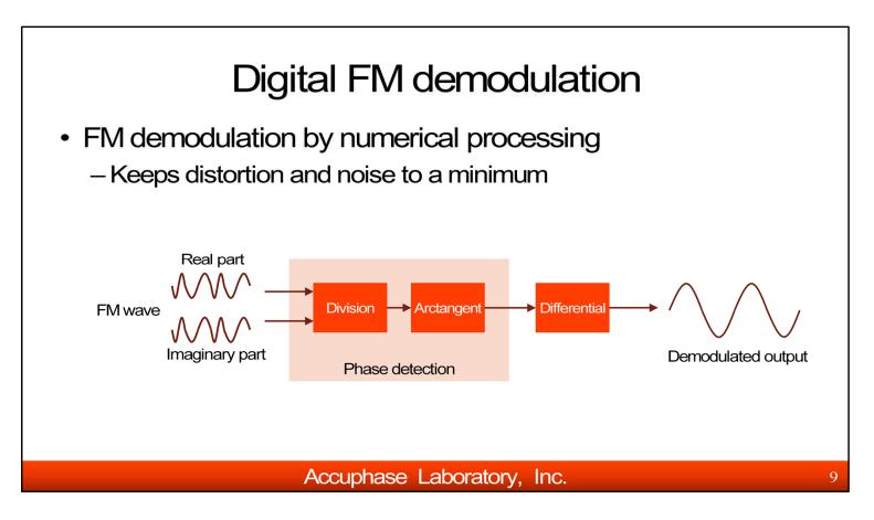
FM demodulator circuit is also based on 40bit floating point DSP chip precisely calculating the theoretical formula to demodulate the FM signal.
