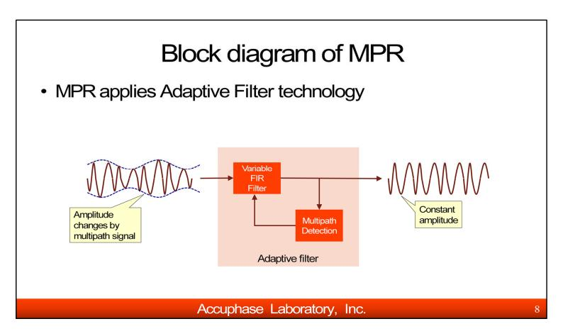
MPR applies the adaptive filter technology that transforms the filter shape to minimize multipath.
