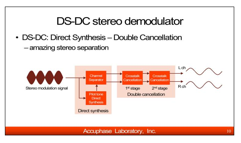
DS-DC is an Accuphase original stereo demodulation technology which achieves amazing stereo separation.
