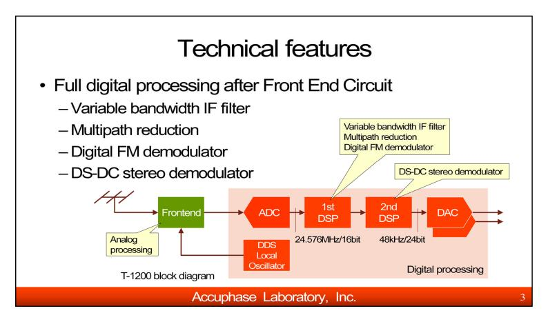
Only the front end which selects and amplifies the weak radio signals is analog circuit. After the front end, all circuits including local Oscillator are digital signal processing.
