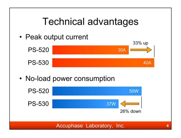
To achieve the enhancement of peak output current and the low output impedance, PS-530 employs bi-polar transistors at power amp block instead of MOS-FET used for PS-520.
