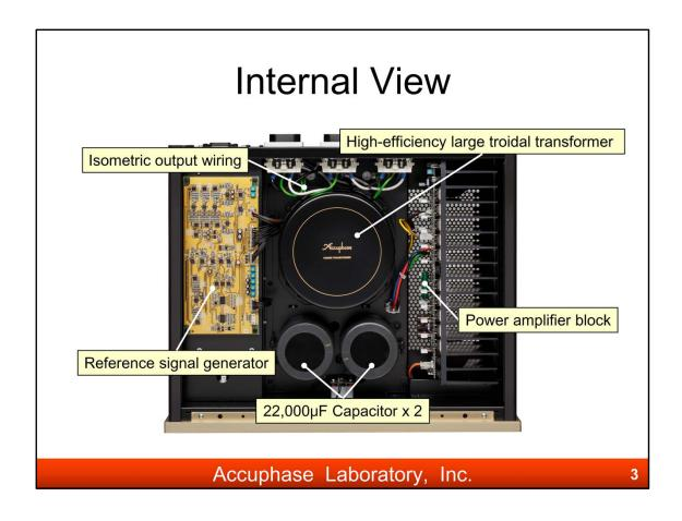
Massive power supply section is arranged at a center position, and power amp block is on right side.
