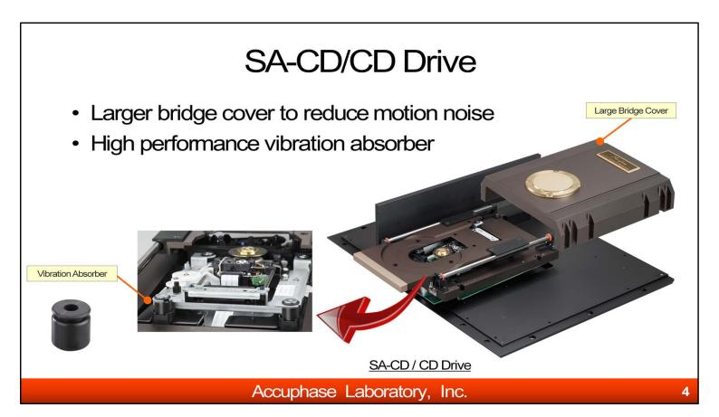
The Bridge cover of SA-CD drive mechanism is bigger and longer than the former model. Outer rotor brushless DC motor is installed at the spindle to drive the discs.
