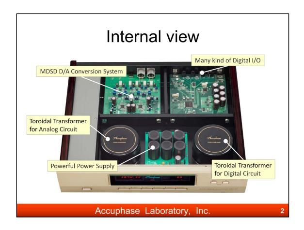
DC-37 has the construction which digital circuit and analog circuit including power transformers are completely separated.
