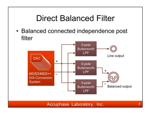
Full-balanced structure is employed after D/A converter in DC-37.
