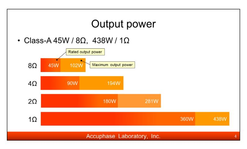
The continuous average output power(rated output power) is 45W into  $8\Omega$  load. However, its actual maximum output power is bigger, saying 102W into  $8\Omega$  and 438W into  $1\Omega$  load.
