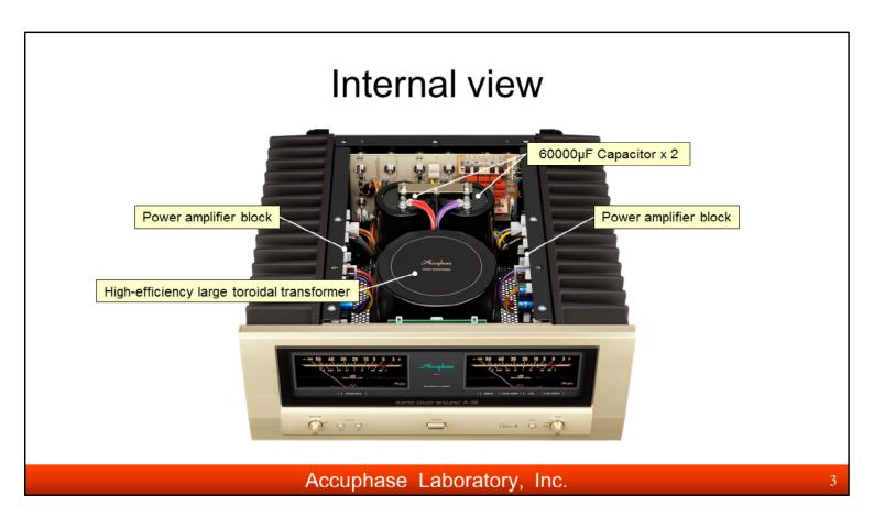
Strong power supply with a massive special made highefficiency toroidal transformer and two large 60000µF special made filtering capacitors are installed.
